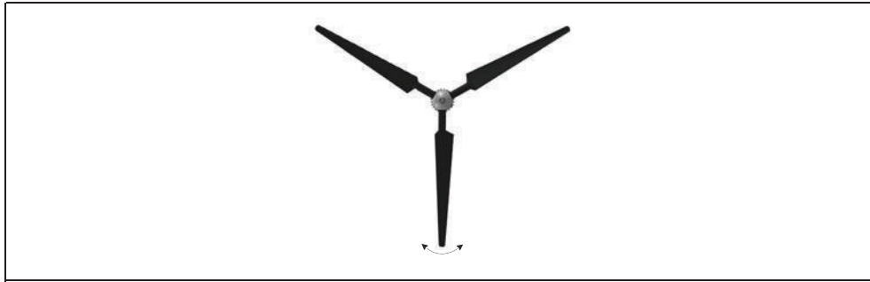
Fig. 7: Balancing the rotor (Y position)
