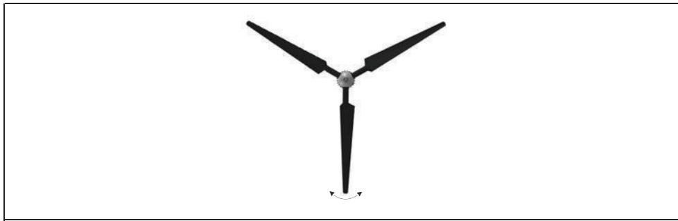
Fig. 7: Balancing the rotor (Y position)
